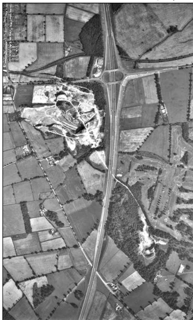
Figure 27. Aerial view of the Charnwood Quarries in 1969. The haul road and conveyor belt pass under the M1 motorway, transporting rock and aggregate between Newhurst (to the northwest) and Longcliffe Quarry (to the southeast). (Photo: Hanson Quarry Products)
